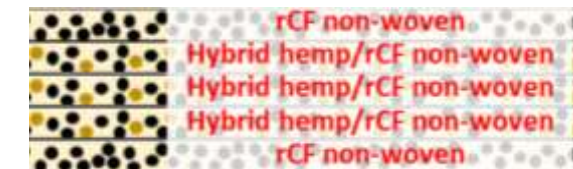
Examples of interply hybrid laminates
