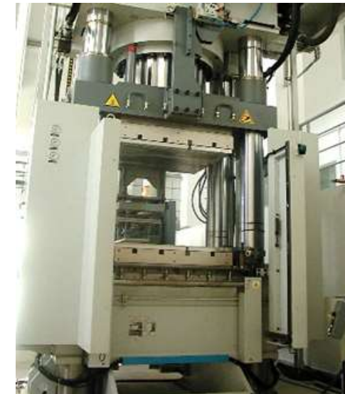
Pilot-scale (CETMA) press for PCM process development
