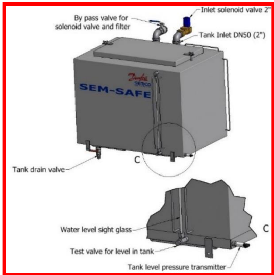
Tank on Unit
