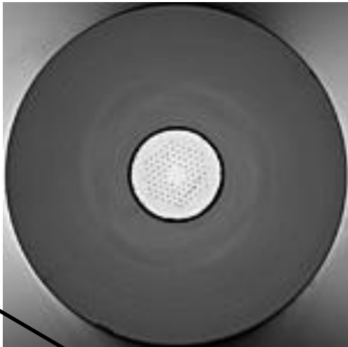
Air-silica microstructured inner cladding
