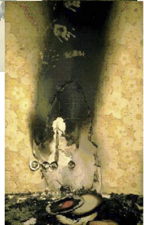
**Antenna line and audio-system damaged by lightning strike**
