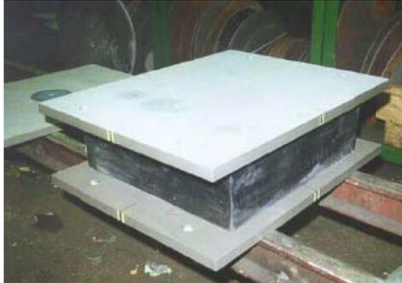
**2** isolatori in gomma armata ad alto smorzamento (**High Damping Rubber Bearing, HDRB**)
