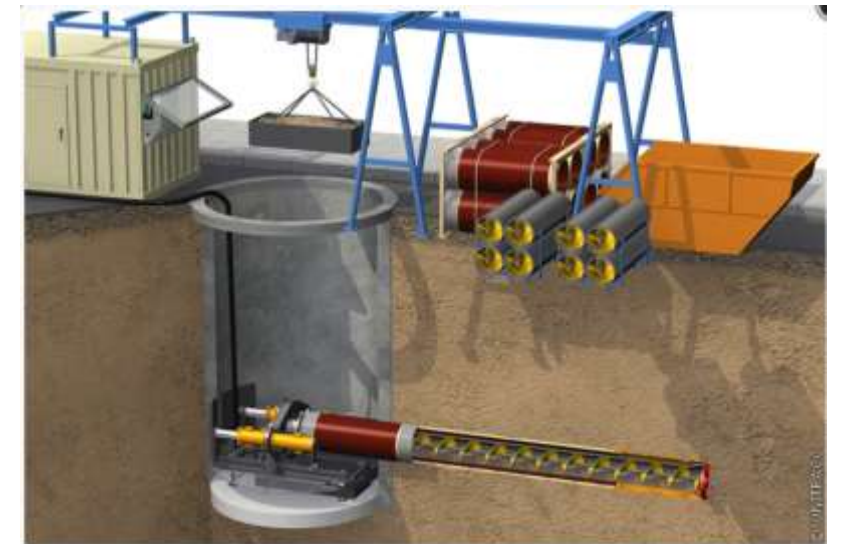
Technical components for microtunneling with auger spoil removal in single phase jacking [Image: S&P GmbH]
