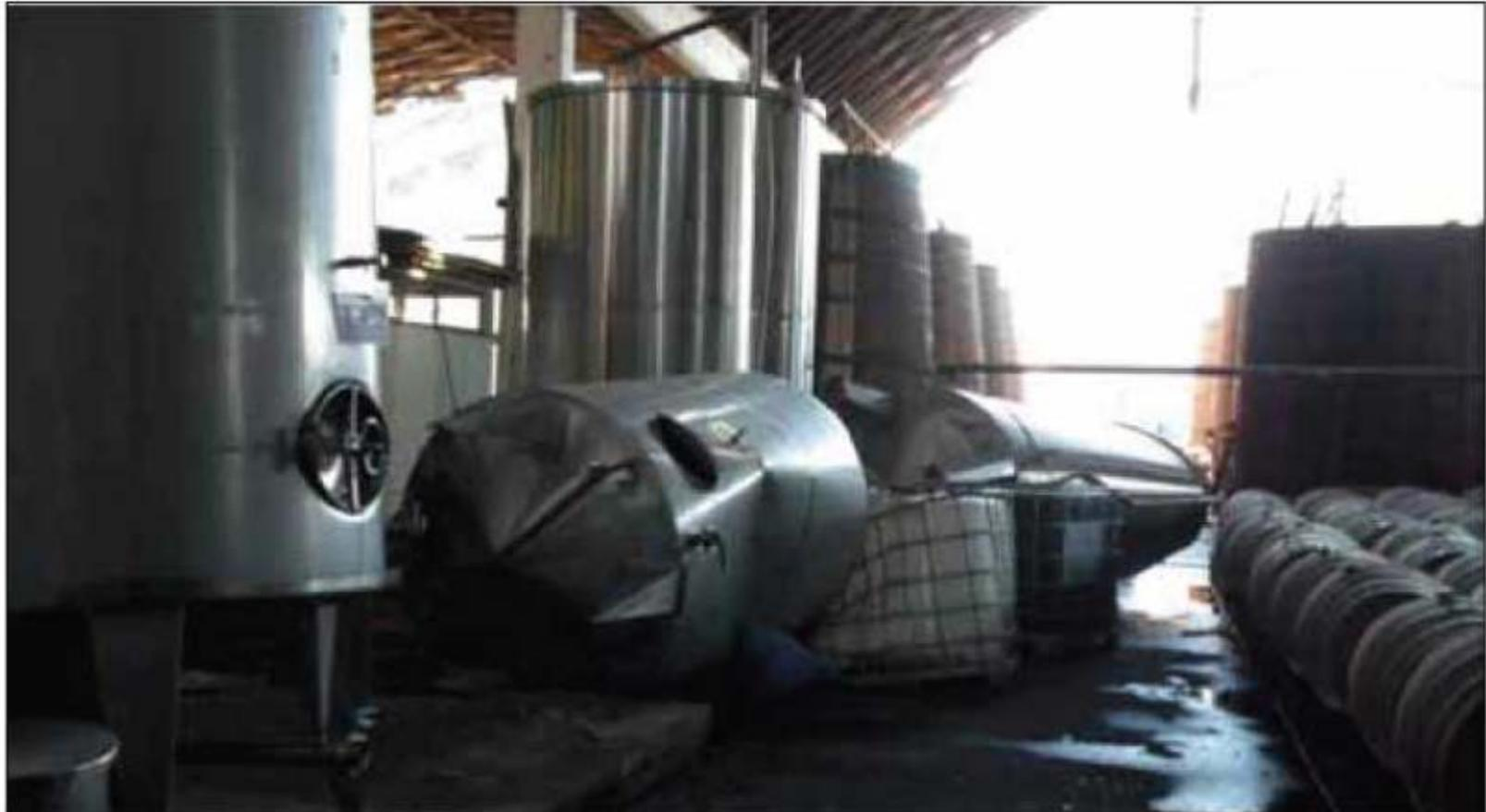
**Figure 28.** *Typical damage to storage tanks in wineries (photo: R. Leon).*
